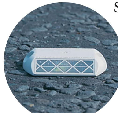
3M 290 studs are classified as being **Type P3A** studs, (i.e. Permanent, Plastic reflector with abrasion resistant layer, non-depressible) and **Class PRP1 Type 2** retroreflectors according to EN1463 part 1:1998. 3M 290 studs achieved the highest possible classifications in road test performance as per EN1463 part 2:2000; **Class S1** (Road Presence) ● **Class R1** (Night-time visibility).
